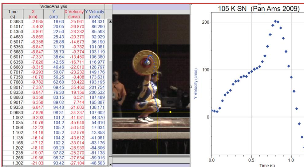
Figure 8. Data Table, Image of the Snatch Catch Position with Bar Trajectory, and Vertical Velocity Graph from the Logger Pro software
