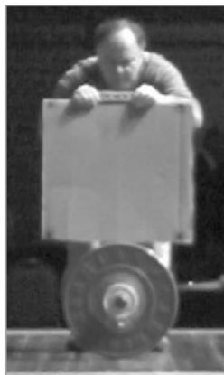
Figure 2. Calibration Using a Square of Known Dimensions
